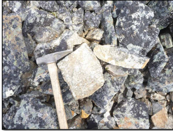
Figure 2: Feldspar porphyritic granodiorite, Rhosgobel Stock
