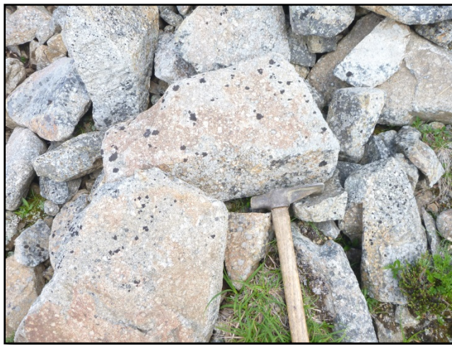
Figure 1: Feldspar porphyritic granodiorite, Pukelman Stock
