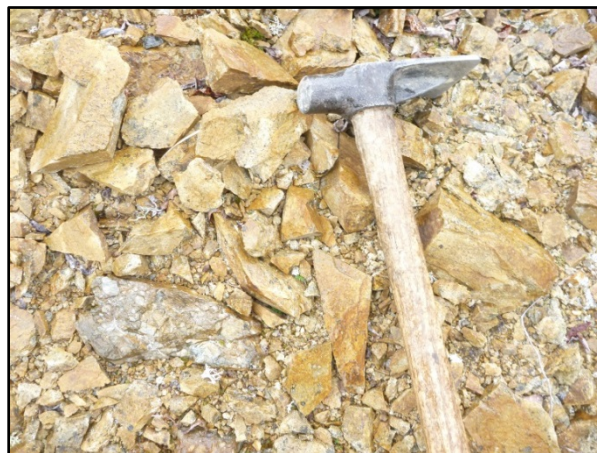
Figure 3: Quartz-Feldspar-Biotite porphyritic monzonite, Bear Paw Zone area
