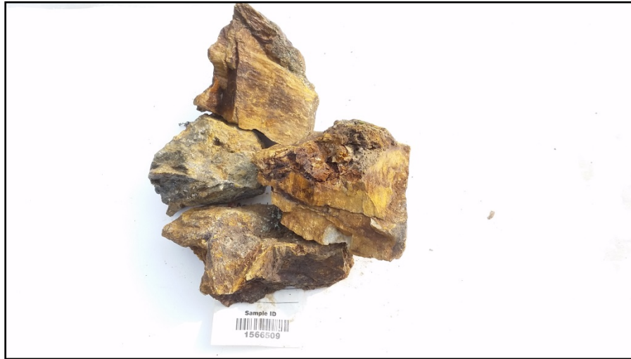
Figure 8: Sample 1566509 (43.4 g/t Au); Qz-As veinlets in phyllite
